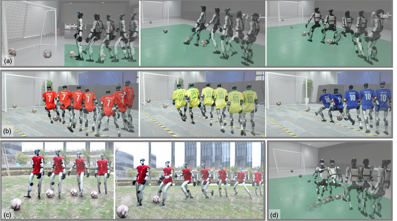
Fig. 1: Humanoid learning soccer skills. (a) The robot performs goal-directed kicks referring to different motions conditioned on the ball position. (b) The robot achieves accurate shots while imitating styles of different professional players. (c) Stable and precise kicking on a grass field. (d) The robot can successfully kick a moving ball.
